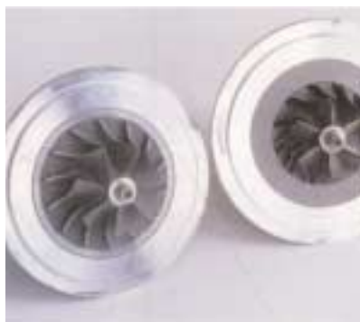
Clockwise from above: Garrett impeller vs. K04 impeller: note difference. APR's optimized exhaust manifold as compared to stocker. K04 vs. Garrett: note housing difference. A4 vs. S4: bet on the lighter 1.8t. APR's S4 exhaust features resonance-chamber technology.
