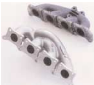
Clockwise from above: Garrett impeller vs. K04 impeller: note difference. APR's optimized exhaust manifold as compared to stocker. K04 vs. Garrett: note housing difference. A4 vs. S4: bet on the lighter 1.8t. APR's S4 exhaust features resonance-chamber technology.
